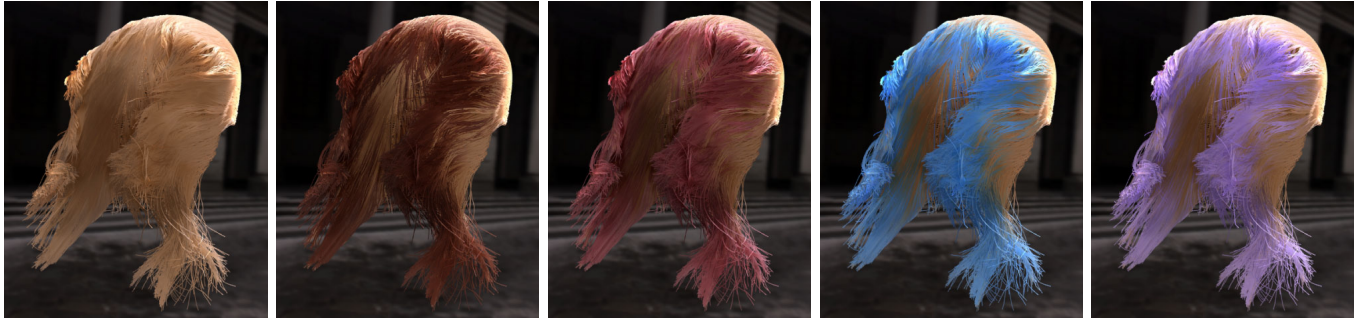
Figure 1: Our algorithm achieves interactive hair rendering and appearance editing under environment lighting, including both single and multiple scattering effects. In this example, the user directly paints onto the hair to edit the spatially-varying scattering parameters. This results in a dynamic simulation of hair coloring. From left to right, the hair is dyed with a progressively more vivid color. The environment map is represented by 40 SRBF lights, and our algorithm runs at 8.3 fps on an NVIDIA GTX 580.
